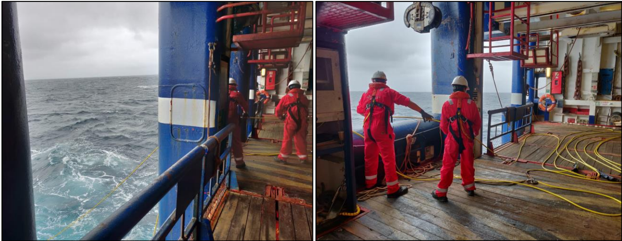
Figure 21 PAM cable being deployed from the stern
