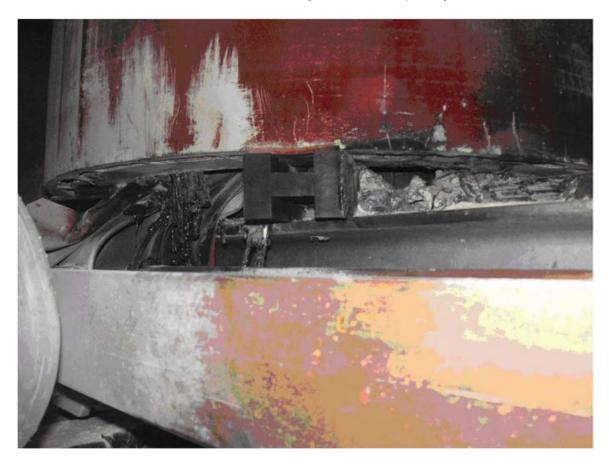
In this incident, the transformers had not been correctly rated. Transformers intended for use with inverter drives should be rated for the additional heating effects imposed by harmonic currents resulting from the non-linear nature of switched and unbalanced loads.
