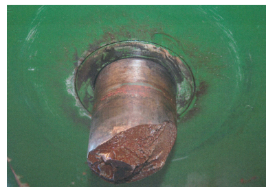
The failed gimbal pin
