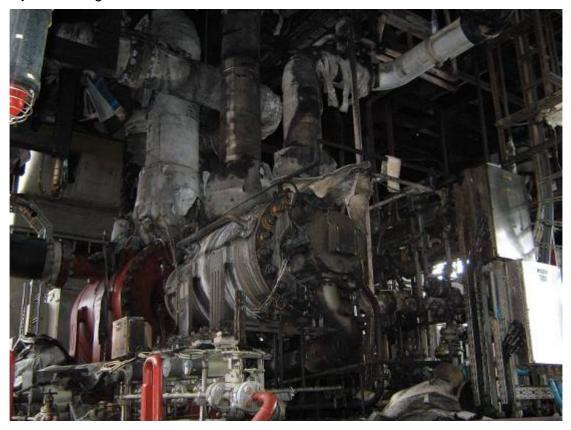
Centrifugal gas compressors are widely utilised on production facilities within Australian waters. They are typically used to compress gas required for export or well re-injection. A typical gas compressor configuration consists of 1<sup>st</sup> LP (low pressure) stage, 2<sup>nd</sup> IP (intermediate pressure) stage and 3<sup>rd</sup> HP (high pressure) stage.
