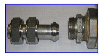
Potential failure will not be evident without adequate post-assembly inspection and may not become apparent for a number of years due to a range of factors including operating conditions and the material of the tube and fittings. Even during regular pressure testing, it is not uncommon for these 'compromised' fittings to pass the initial and subsequent tests prior to the main failure event.
