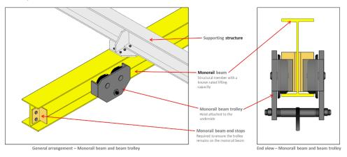
NOPSEMA deployed inspectors to the facility to investigate. Preliminary findings identified that the lifting system (end-stops / trolley / rail) were not fit for purpose. The trolley had been modified outside of management of change processes and the lift plan was not followed, resulting in unsafe operation of the chain hoist.
