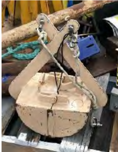
Figure 8 Van Veen grab sampler. Provided by Fugro, March 2020.
